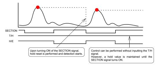
However, when the auto reset functions, if the signal causes chattering, the point that should be taken originally may deviate. Switching is provided so as to prevent the next detection from being performed until the T/H signal is turned on even if the SECTION signal is turned on again.
